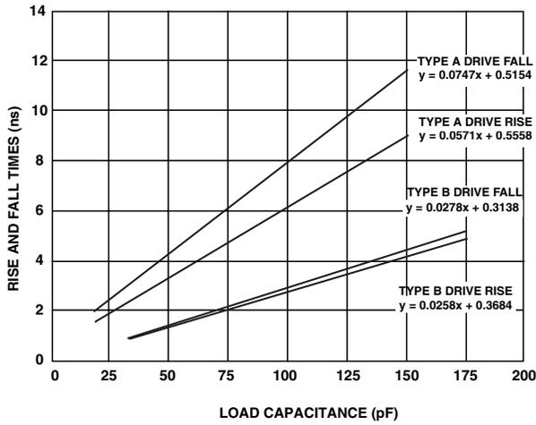
Figure 45. Typical Output Rise/Fall Time
