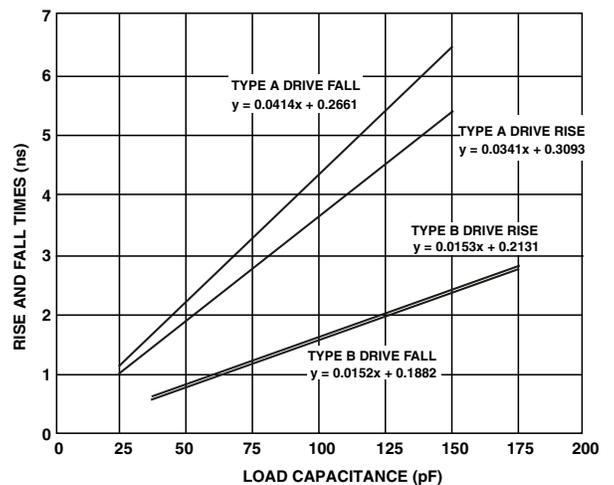
Figure 44. Typical Output Rise/Fall Time (20% to 80%,  $V_{DD\_EXT} = \text{Max}$ )
