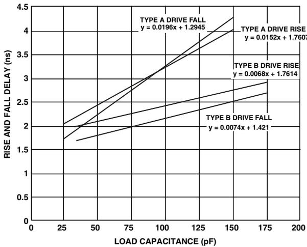
Figure 46. Typical Output Rise/Fall Delay
