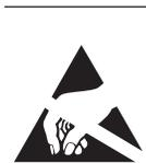
**ESD (electrostatic discharge) sensitive device.** Charged devices and circuit boards can discharge without detection. Although this product features patented or proprietary protection circuitry, damage may occur on devices subjected to high energy ESD. Therefore, proper ESD precautions should be taken to avoid performance degradation or loss of functionality.
