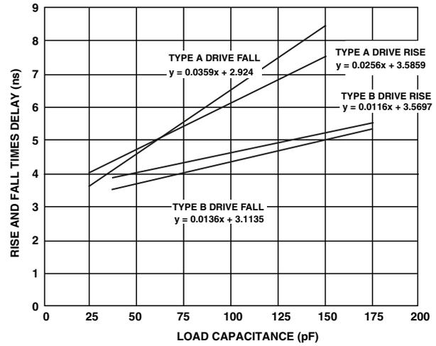
Figure 47. Typical Output Rise/Fall Delay
