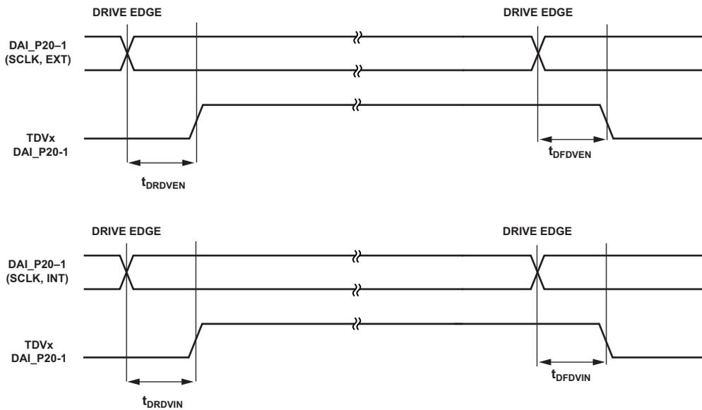
Figure 24. Serial Ports—TDM Internal and External Clock
