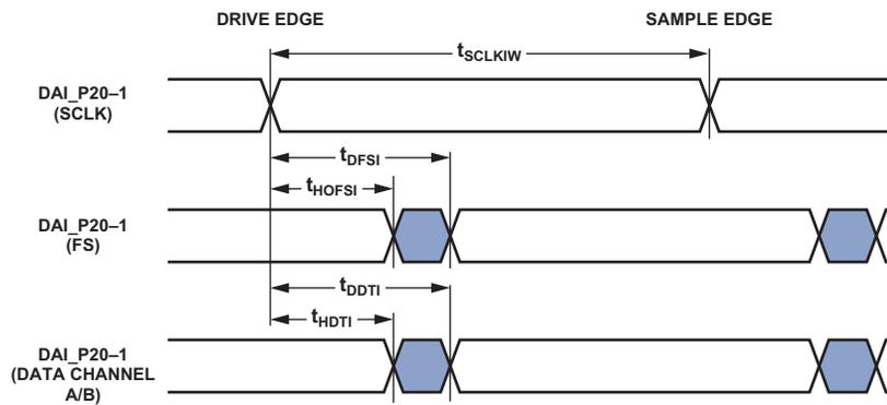
Figure 34. S/PDIF Receiver Internal Digital PLL Mode Timing
