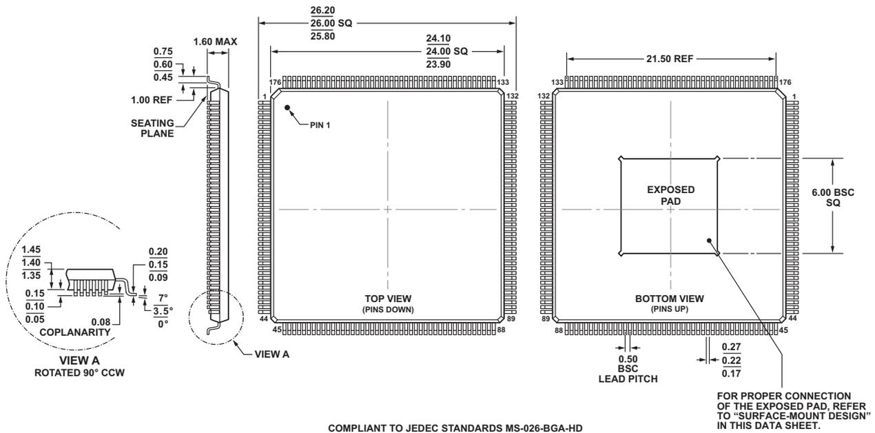
Figure 53. 176-Lead Low Profile Quad Flat Package, Exposed Pad [LQFP\_EP]<sup>1</sup>
