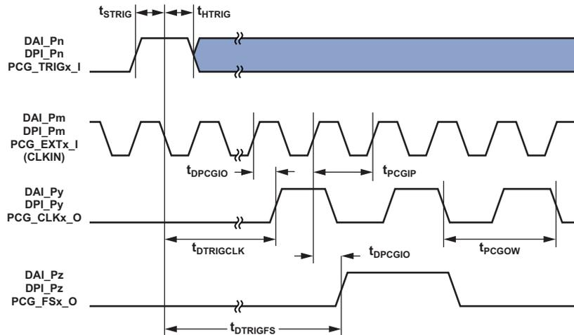
Figure 16. Precision Clock Generator (Direct Pin Routing)
