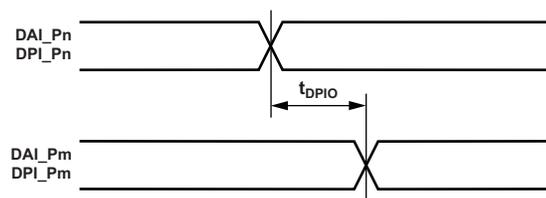
Figure 15. DAI Pin to Pin Direct Routing
