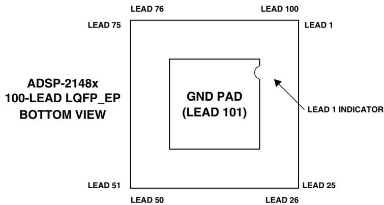
Figure 49. 100-Lead LQFP\_EP Lead Configuration (Bottom View)
