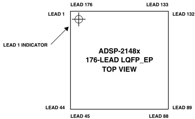
Figure 50. 176-Lead LQFP\_EP Lead Configuration (Top View)
