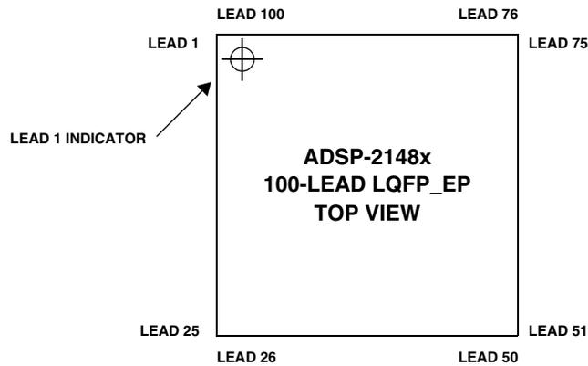
Figure 48. 100-Lead LQFP\_EP Lead Configuration (Top View)
