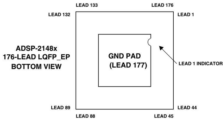
Figure 51. 176-Lead LQFP\_EP Lead Configuration (Bottom View)
