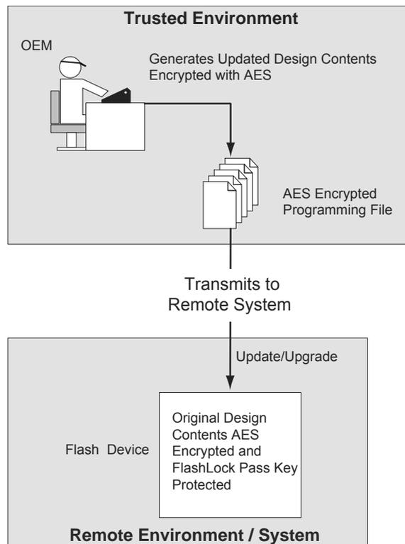
Figure 12-8 • Application 3: Nontrusted Environment—Field Updates/Upgrades
