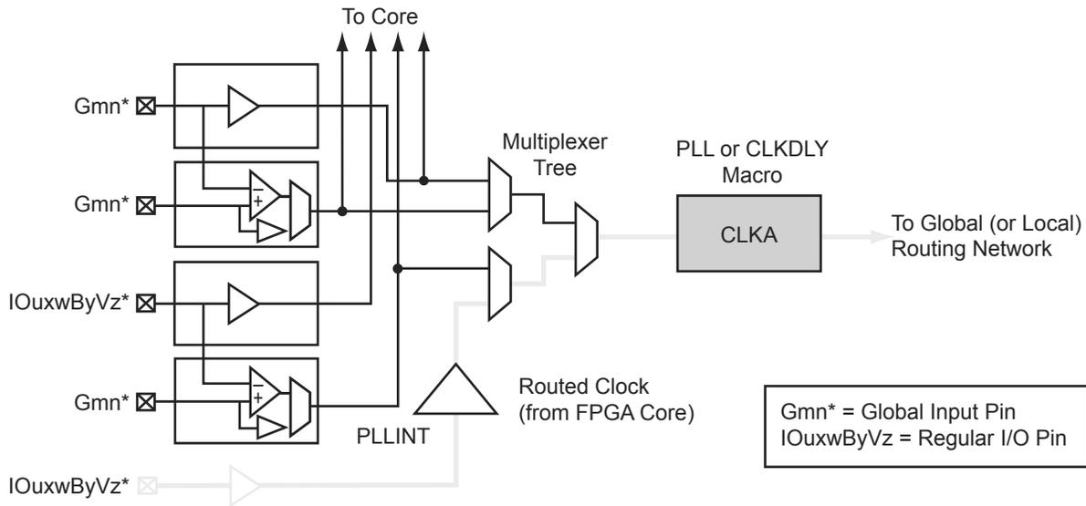
**Figure 4-11 • Illustration of External I/O Usage**
