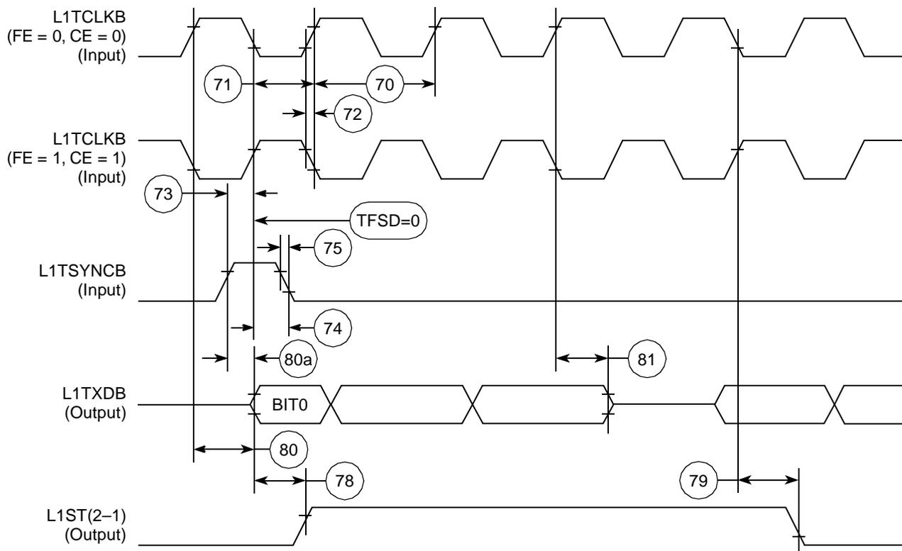
Figure 50. SI Transmit Timing Diagram (DSC = 0)
