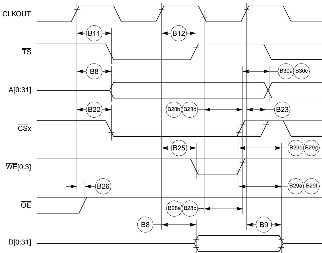
Figure 17. External Bus Write Timing (GPCM Controlled—TRLX = 0, CSNT = 1)
