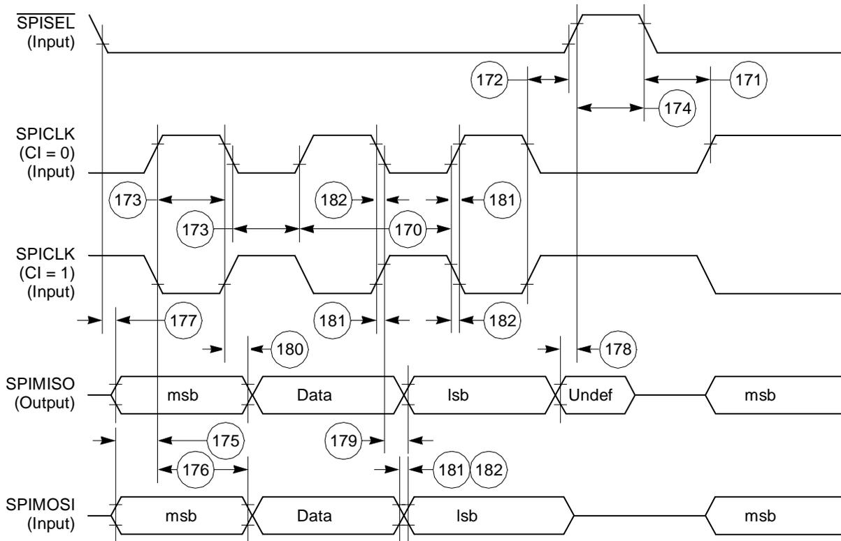
Figure 62. SPI Slave (CP = 0) Timing Diagram
