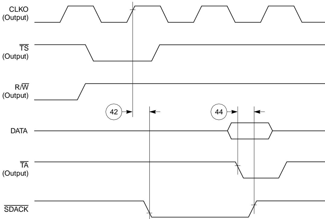
Figure 44.  $\overline{\text{SDACK}}$  Timing Diagram—Peripheral Write, Internally-Generated  $\overline{\text{TA}}$
