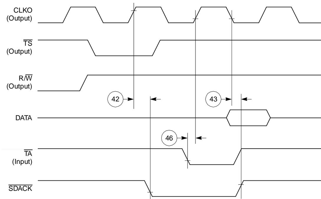
Figure 43.  $\overline{SDACK}$  Timing Diagram—Peripheral Write, Externally-Generated  $\overline{TA}$
