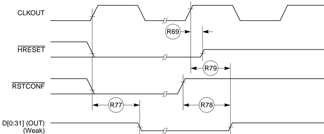
Figure 35. Reset Timing—Data Bus Weak Drive During Configuration
