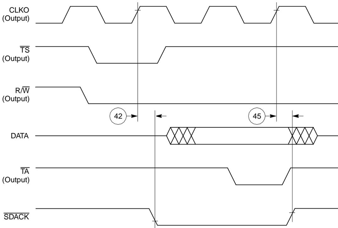
Figure 45.  $\overline{\text{SDACK}}$  Timing Diagram—Peripheral Read, Internally-Generated  $\overline{\text{TA}}$
